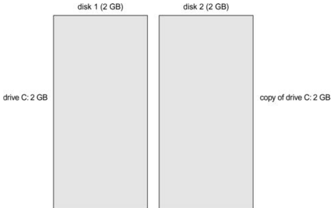
Figure C.10 Mirror set on two drives.
